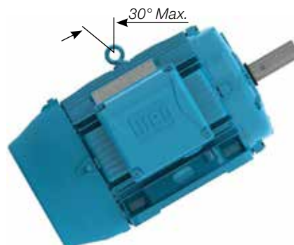
Figure 4.3 - Maximum allowed angle-of-inclination for motor with one eyeboll
