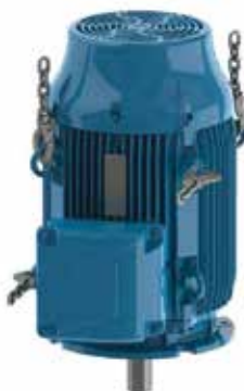
Figure 4.17 - Install the second pair of eyebolts
