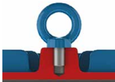
Figure 4.1 - Correct tightening of the eyeboll
