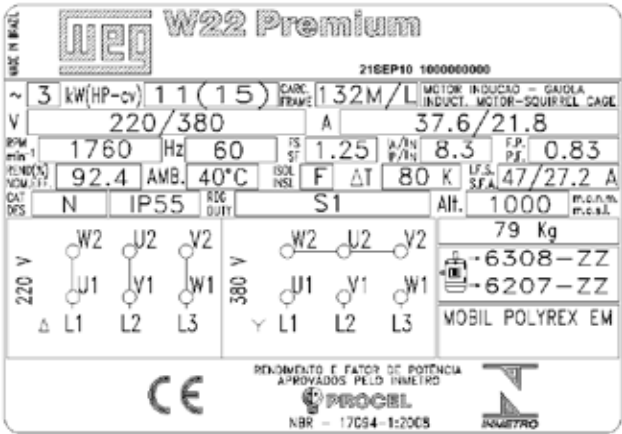
Figure 2.1 - IEC motor nameplate
