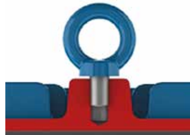
Figure 4.2 - Incorrect tightening of the eyeboll
