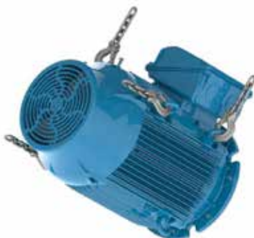
Figure 4.18 - Motor is being rotated to horizontal position
