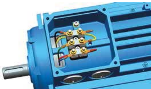
Terminal board for motor sizes 71-80.
