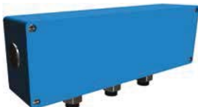
Large auxiliary aluminum terminal box for motor sizes 280-450. The size of terminal box ordered with these codes depends on the number of accessories ordered. 80 x 250 mm, max 30 strips. Earthing size M4
