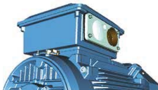
Terminal box for motor sizes 160-250. Connection flanges with tapped cable entries.
