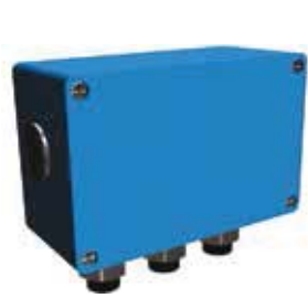
Small auxiliary aluminum terminal box for motor sizes 280-450 (variant codes 418, 568, 380, 569) The size of terminal box ordered with these codes depends on the number of accessories ordered. 80 x 125 mm, max 12 strips. Earthing size M4
